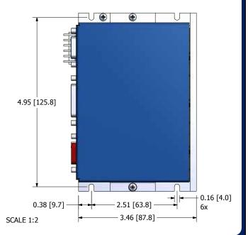
Download STP solid model of this electronics module here: http://www.tecnadyne.com/rotary\_actuators
